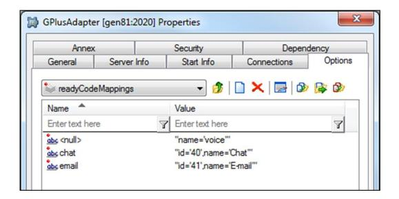
The id field can be either the new RTA State Name or State ID as defined in the <u>RTA State table</u>. The name field is the new Reason that will be included with the RTA state message sent to the WFM server.
