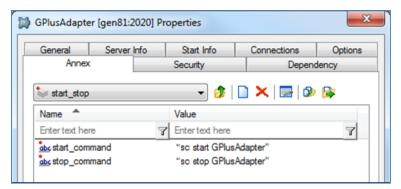
The sc command is the Windows Service Control application and it is used to either start or stop the Adapter service.
