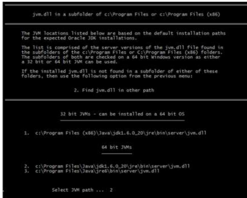
The change is immediately written to the config\jvm.properties file and the status section reflects the specification of the 64 bit JVM as shown below.
