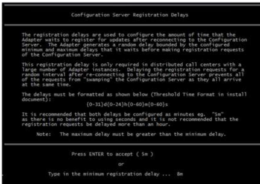
As mentioned, the response from the Configuration Server can be significantly delayed in very busy call centers. The registration timeout option sets the amount of time that the Adapter will wait before generating a new request.
