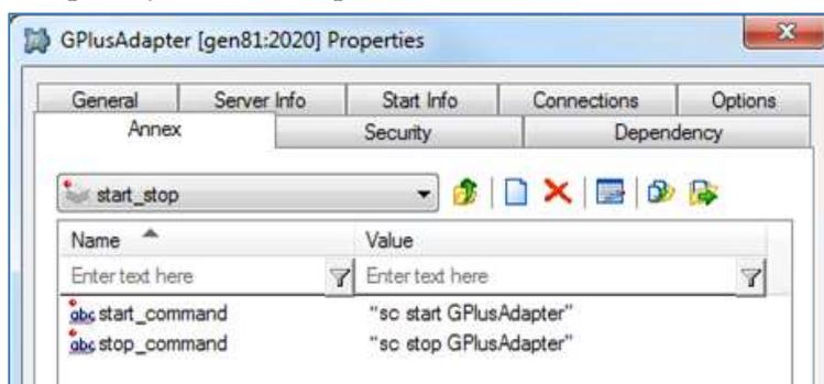
Adapter instance. The example below shows the configuration for a Service instance named GPlusAdapter.
