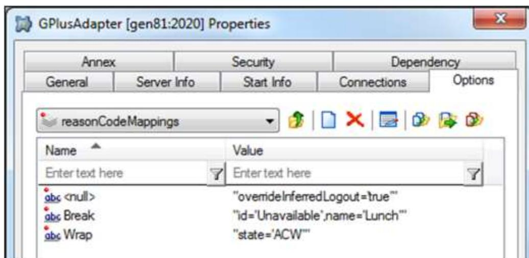
The id field can be either the new RTA State Name or State ID as defined in the [RTA State table](#). The name field is the new Reason that will be included with the RTA state message sent to the eWFM server. The state field allows the event to be interpreted as either Unavailable or ACW in the historical reports.
