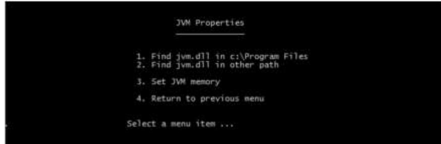
There are two different menu options for finding the path to the jvm.dll file. The first just looks in the default locations that the Oracle installation application will place a 32 bit or 64 bit version while the second option allows a path to be set with all of the subfolders being searched.
