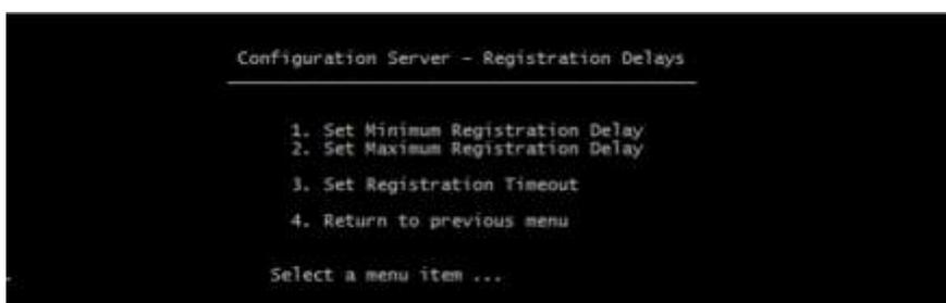
The registration delays are the minimum and maximum bounds of the time that the *Gplus* Adapter will wait before making a registration request of the Configuration Server after the connection has been restored. The Adapter will wait a random time between the two limits.
